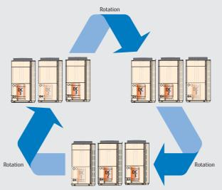
Note: Rotational operation is alternated by the start / stop timing of the compressor.
