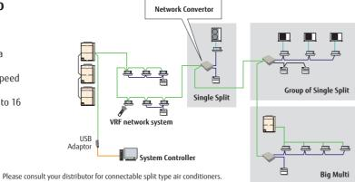
Up to 100 Network Convertors may be connected in a single VRF network system. One Network Convertor is considered as a single refrigerant system, irrespective of the number of connected single models.
