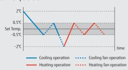
The auto change over setting allows for the product to easily switch between the cooling and heating modes regardless of the operation mode of the other indoor units. This can be done via a specific indoor unit with wired remote controller. This ensures comfortable operation all year round.
