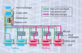
Our heat recovery systems can achieve high operating energy efficiency by drawing heat from the room to be cooled and transferring it as energy for rooms that are to be heated.
