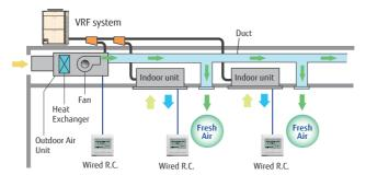
\* Make sure the connected capacity is within the range of 50% to 100% of the outdoor unit capacity. In addition, if there are mixed connections with indoor units, the Outdoor Air Unit connection capacity becomes 30% or less of the outdoor unit capacity.
