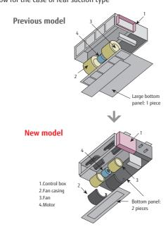
Structural improvement is attained by making the bottom panel two pieces, front and rear. The internal fan casing is also manufactured in two pieces, namely upper and lower. The maintenance of the motor and fan can be easily carried out by removing the rear panel and the lower part of the casing while leaving the main chassis installed.
